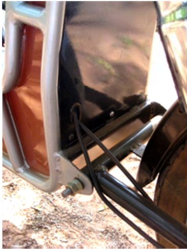
Wires connecting to motor and brake
