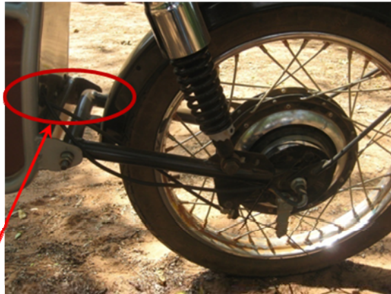
Wires connecting to motor and brake
