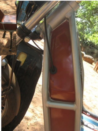
Rear brake wire running through the body
