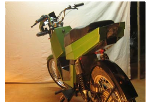
Tail light – integration of Bajaj XCD LED light
