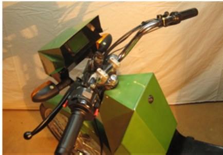
Digital speed and battery indicator
