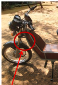
Rear brake wire running through the body
