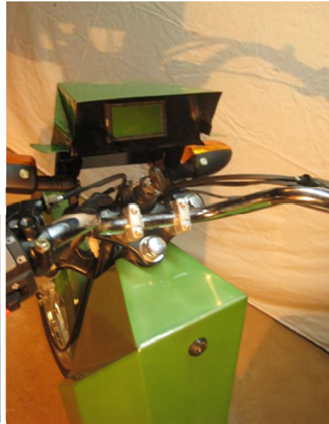
Digital speed and battery indicator
