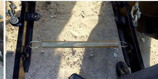
HYDRAULIC ARM SPRING LINK (FREE FROM INCONVENIENCE DUE TO SHACKLE)
