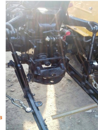
HYDRAULIC ARM SPRING LINK (FREE FROM INCONVENIENCE DUE TO SHACKLE)
