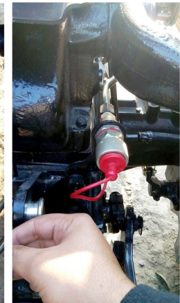
BUILT IN OUTLET FOR PRESSURE TROLLEY , EASY MAINTENANCE, RAPID CONNECTION WITH TROLLEY HOSE
