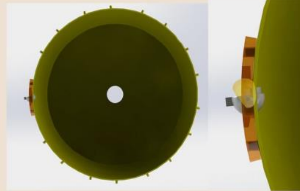
Step 2 : As the drum rotates (anti clockwise) ,the seed is isolated by the cap mechanism.
