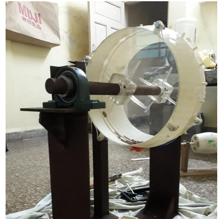
3D printed seed drum with acrylic lids
