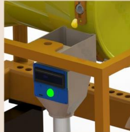
Step 4 : Seed is dropped into the indicator + counter, and the cycle starts all over again.
