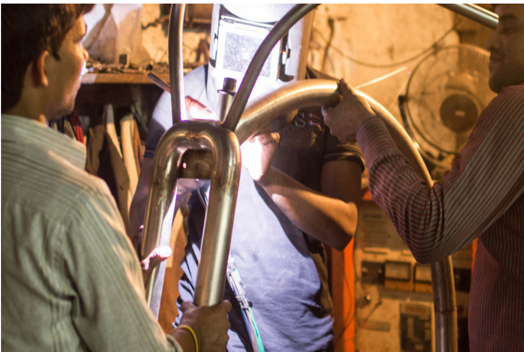
■ Top tube welding
