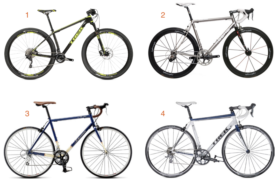
Fig 9. 1. Carbon fibre 2. Titanium 3. Steel 4. Aluminum
