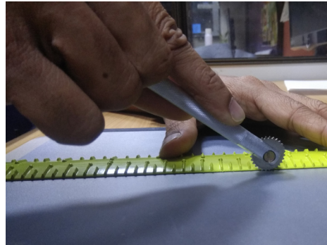
Fig 64. thickness of the scale is more than the radius of spur wheel
