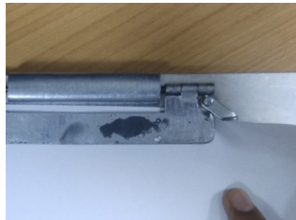
Fig 49. Inconvenience in locking the clip.
