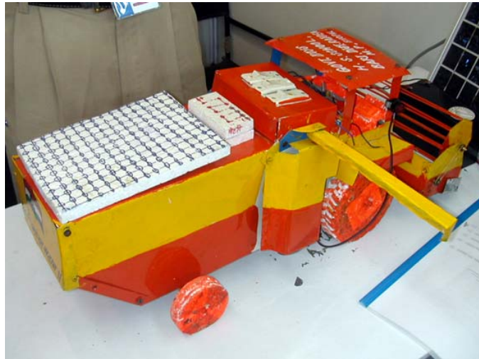
Model of a Solar powered harvester made with plywood platform and aluminium sheet body. Materials like nails and screws were used for joinery. Battery power was used to simulate the power generated by the solar panels mounted on the body of the harvester. The model was made by a X class student.
