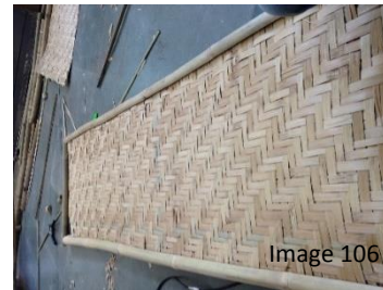
Bamboo mat attached in the slit bamboo frame
