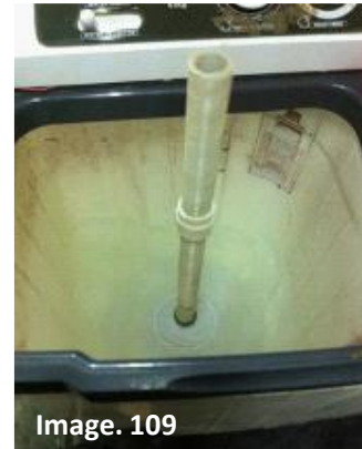
Image. 109 Shaft attached to pulsator causing good water turbulence
