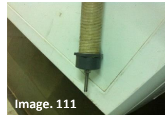
Image. 111 End cap out on base of shaft for smooth rotation
