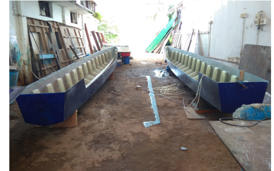
Both hulls trimmed and ready for assembly
