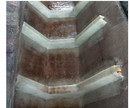
Ribs are packed with PU-foam blocks for strength
