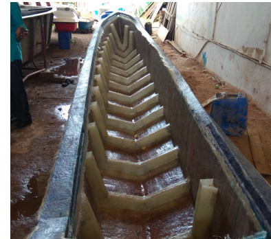
Ribs laid into the hull
