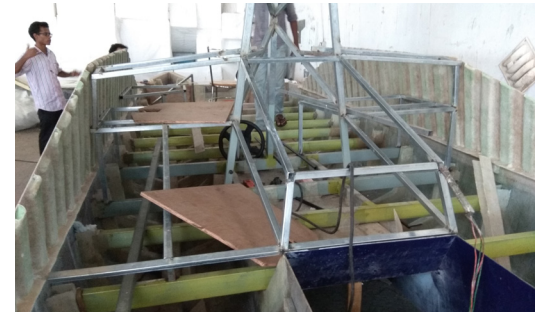
Battery box and seating framework being setup
