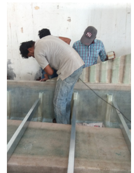
Backrest being bolted onto the hull
