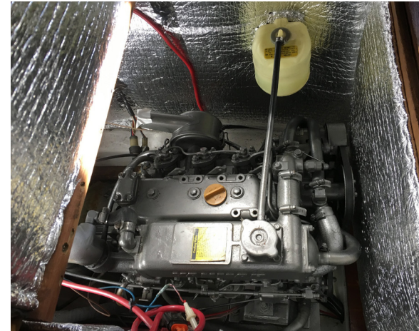
Yanmar inboard diesel engine with sound damping cabin
