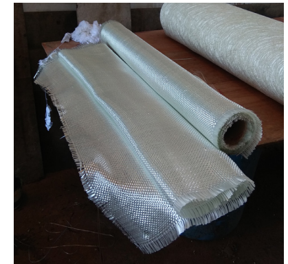
Woven mats cut up and kept ready for laying
