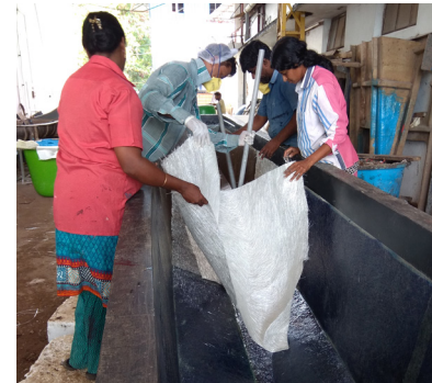
Fibre mats being laid into the mould
