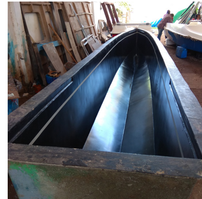
A cleaned mould with the releasing agent applied inside
