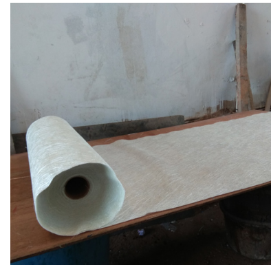
A roll of chopped strand mat being prepped for laying
