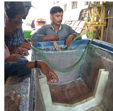
Water being filled to release the hull piece
