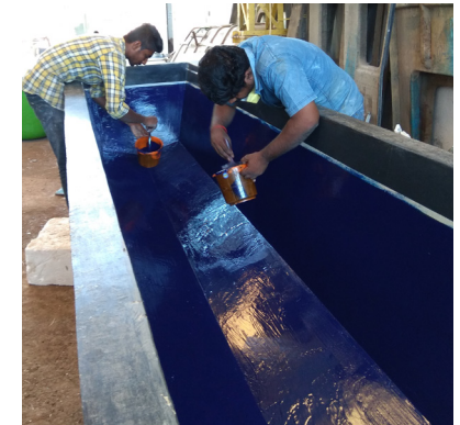
Blue gel coat being applied in the mould for colouring the hull
