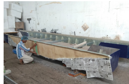
Hull being used as the mould for the backrest
