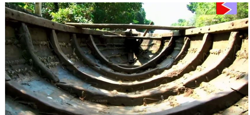
Img 17. Ribs which hold the basic structure of the boat together
