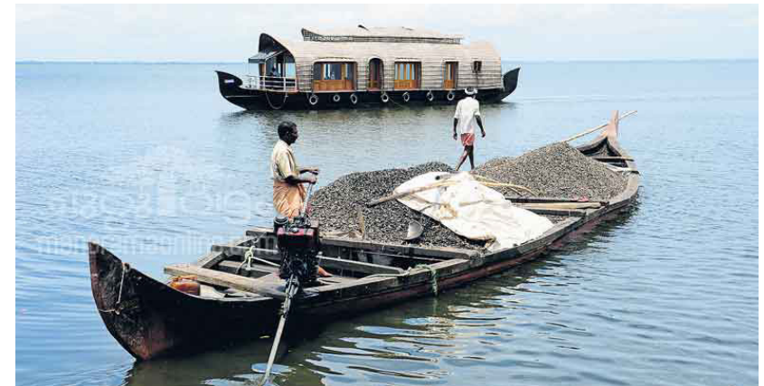
Img 14. A traditional kevuvallam retrofitted with an outboard motor
