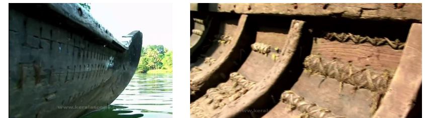
Img 15, 16. Details of kevuvallam. Sewing patterns can be seen
