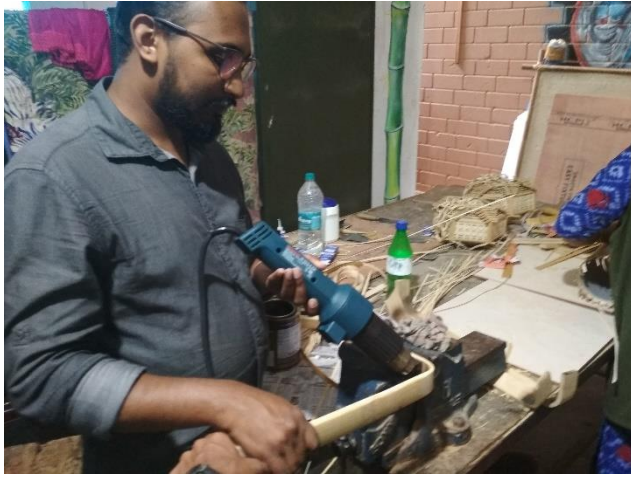
Bending the reapers using hot air gun
