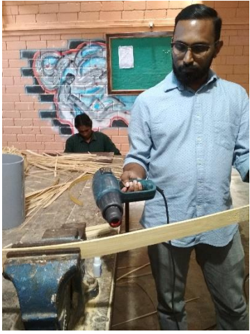
Bending the reapers using hot air gun
