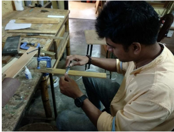
Scraping the surface of the gigantus bamboo reapers using a knife
