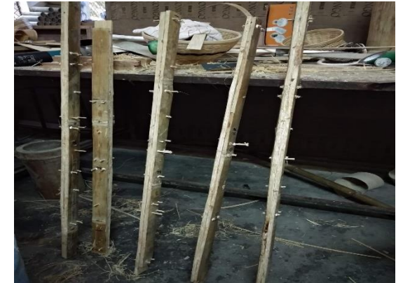
Sticking and nailing two one-side reapers to make leg pieces
