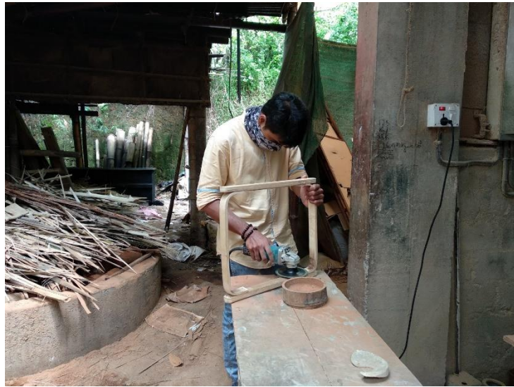
Finishing the frame using an angle grinder
