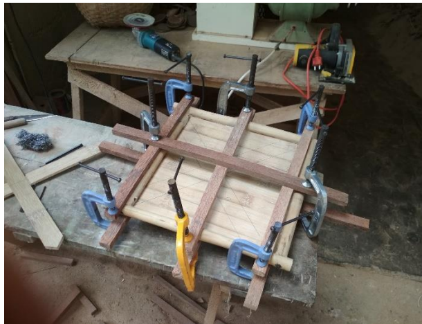
Assembling the seat piece to the strictus frame
