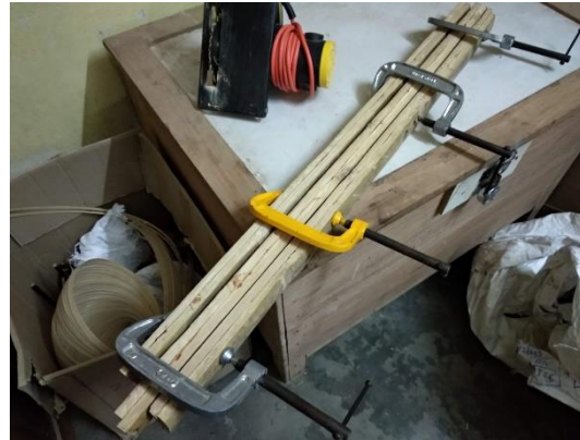
Sticking and nailing two one-side reapers to make leg pieces
