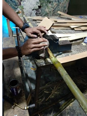
Straightening the strictus pieces using an LPG blow torch
