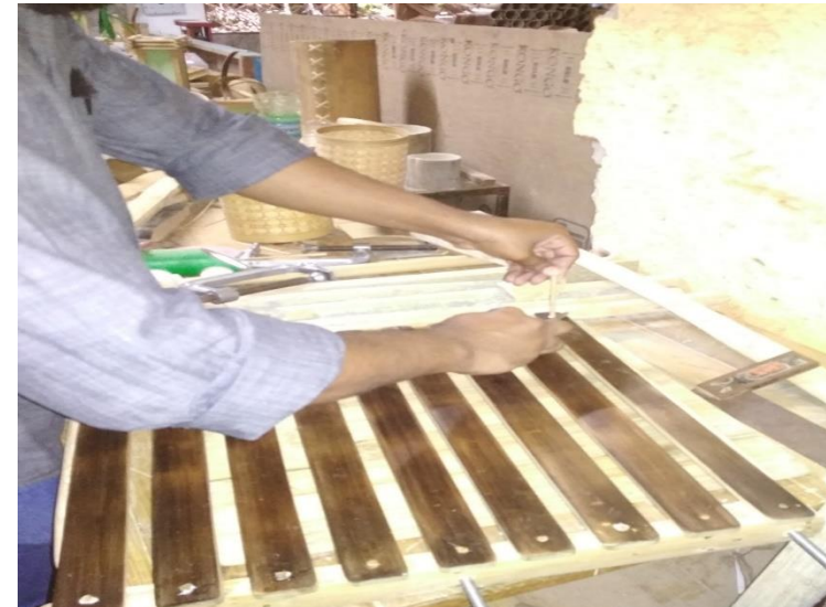
Nailing the seat panels to the frame
