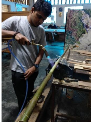
Straightening the strictus pieces using an LPG blow torch
