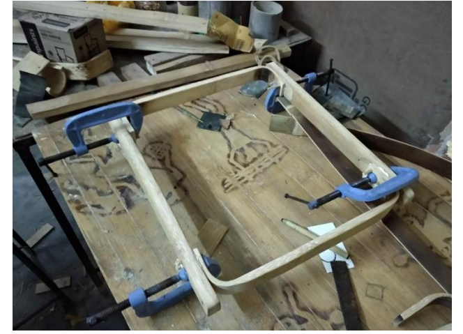
Assembling the seat frame
