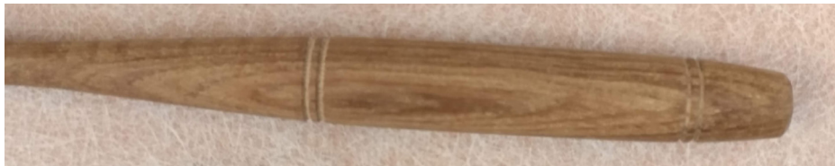
Figure 78. 2 v-grooves on both the side of the handle
