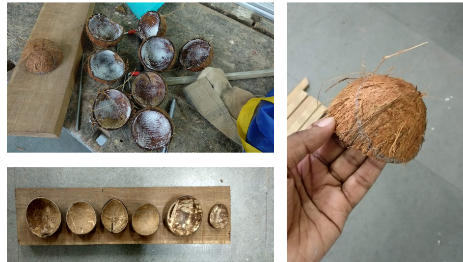
Figure 67. Obtaining usable shapes from discarded coconut shells
