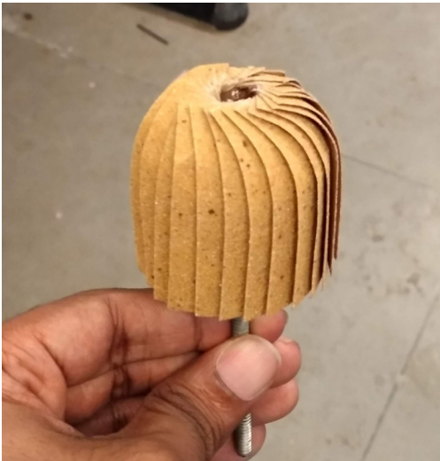
Figure 94. Sanding bit for sanding the inside of the coconut shell
