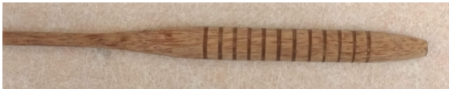
Figure 80. Rectangular grooves at an interval with silicon filling
