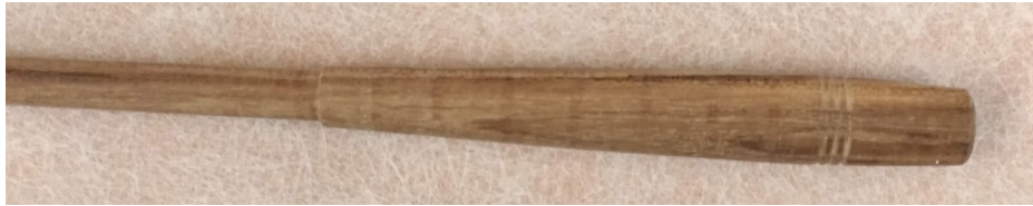
Figure 76. 3 v-grooves on one end and a step on the other end of the handle
