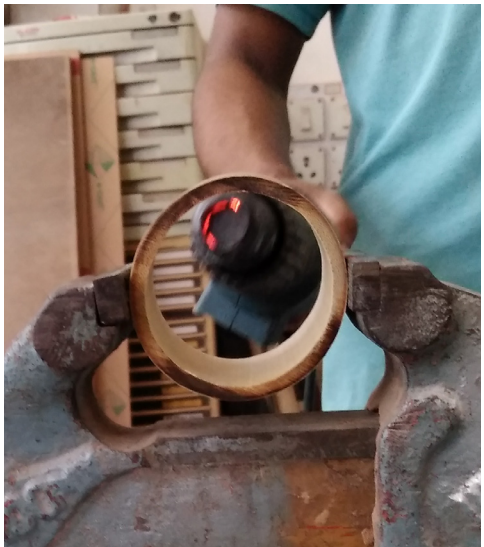
Fig 131. Correcting the roundness of the bamboo by using a hot air gun and bench vice.
