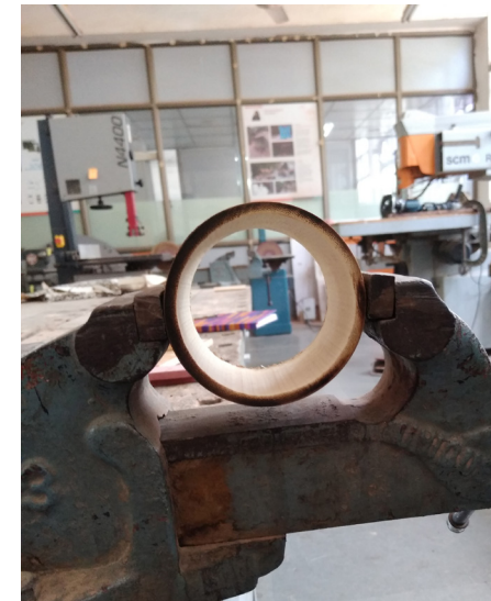
Fig 131. Correcting the roundness of the bamboo by using a hot air gun and bench vice.
