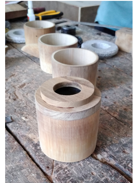
Fig 132. Making the wooden parts for the top piece and attaching it to the bamboo piece.
