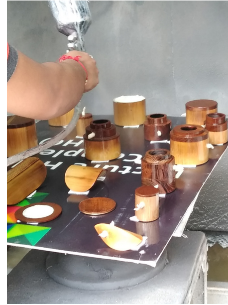
Fig 139. Applying melamine spray polish
