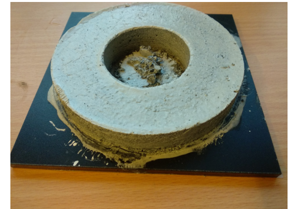
Fig 140. Casting the concrete base
