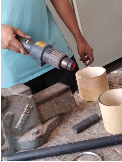
Fig 130. Creating a gradient by burning the surface using a hot air gun
