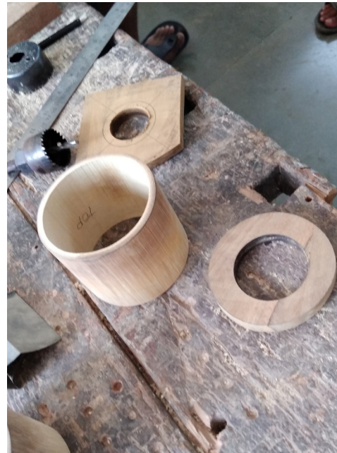
Fig 132. Making the wooden parts for the top piece and attaching it to the bamboo piece.
