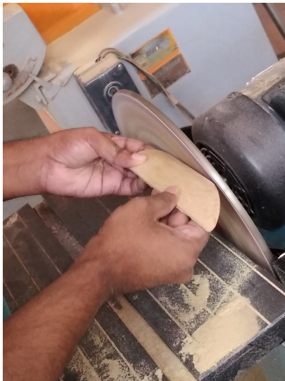
Fig 129. Removing the outer layer by using a sanding machine
