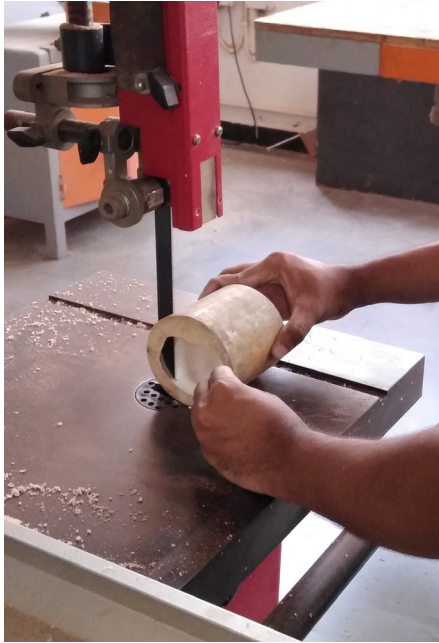
Fig 128. Cutting the bamboo piece to the required size
