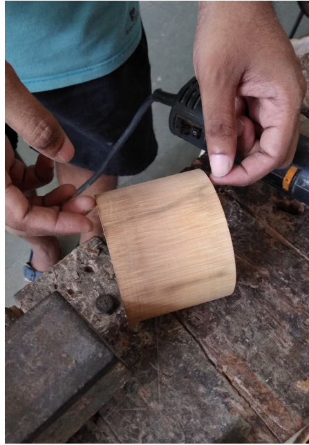
Fig 130. Creating a gradient by burning the surface using a hot air gun
