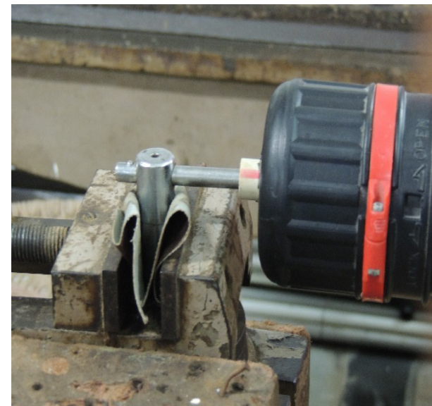
Fig.95: Temporary fixing other end of shaft for stationary operation
