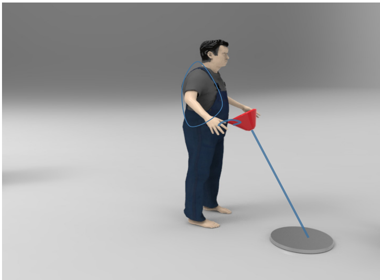
Fig.103: Pros: Manoeuvrability, Sweeping/ Mowing action possible Cons: Vibrational fatigue in the hands
