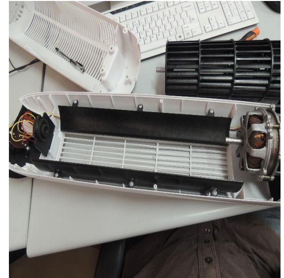
Fig.87: Shroud of tower fan
