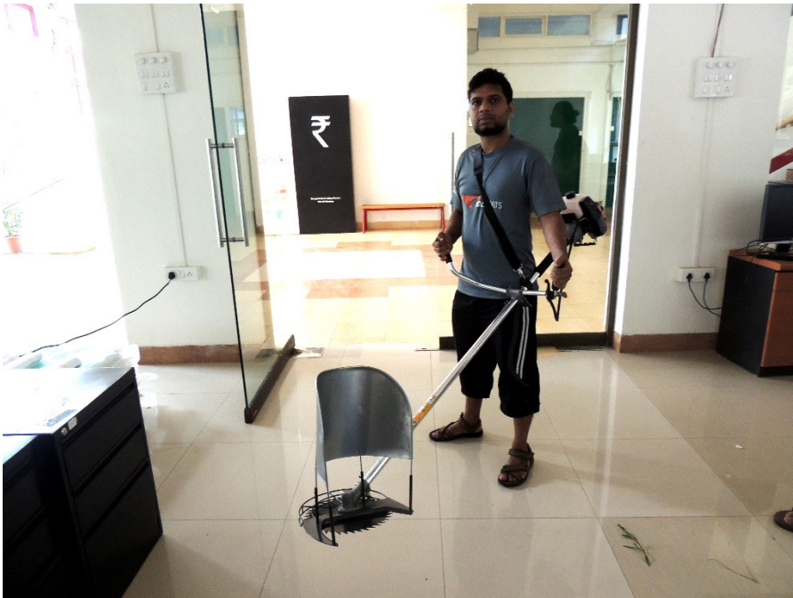
Fig.73: Paddy harvester body worn
