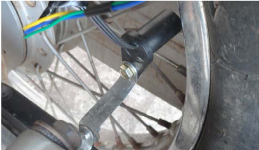
Figure 1. Hall effect sensor installation
