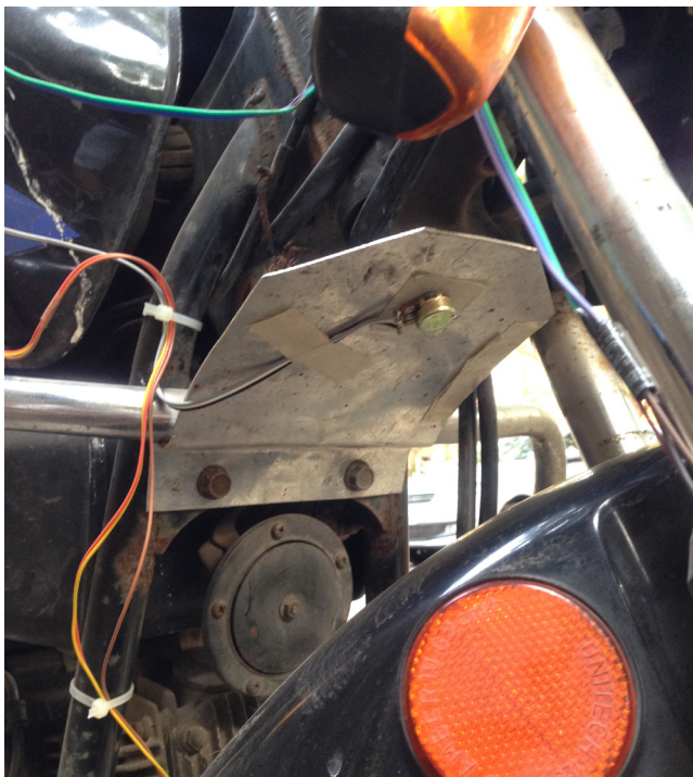
Figure 17. Potentiometer (top) and its installation in Bike
