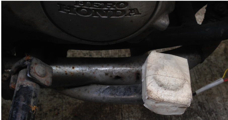
Figure 15. Pressure sensor and its installation on Bike
