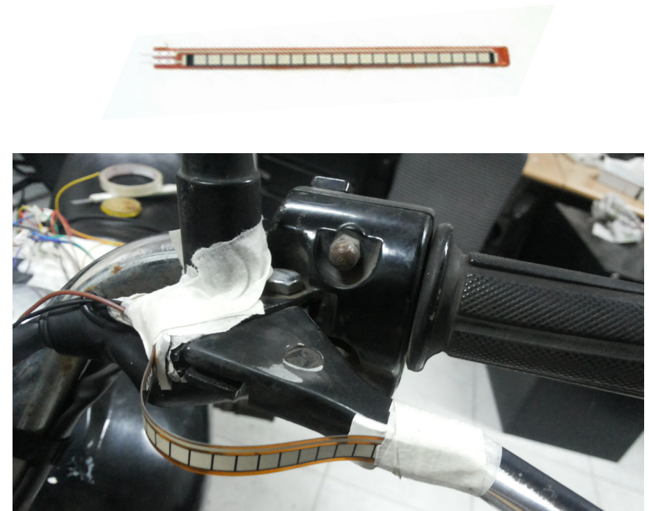
Figure 14. Flex sensor (top) and its installation
