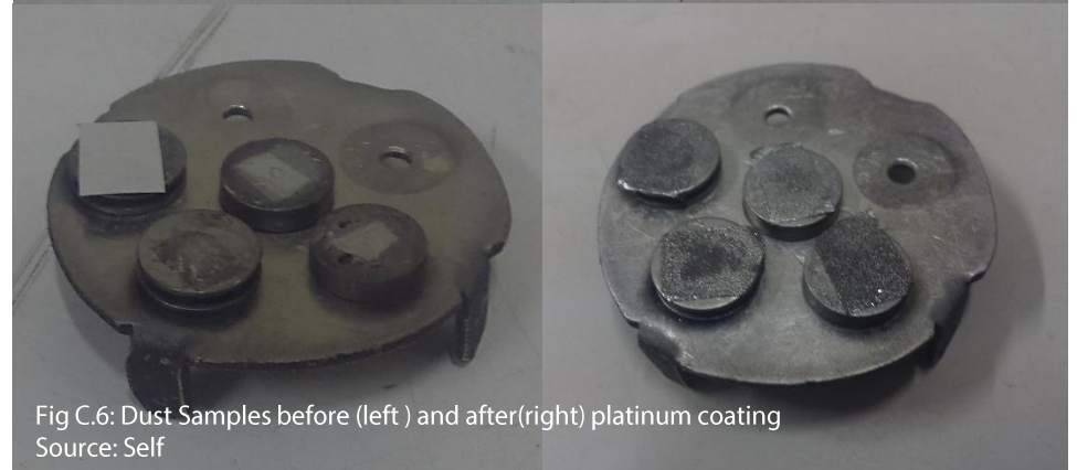
Fig C.5: Collected dust samples are prepared, adhered to the carbon tape for platinum coating. Source: Self
