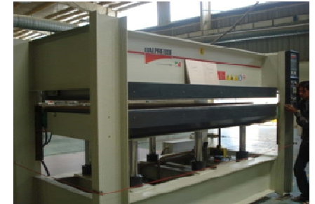
Pressing of board after application of veneer
