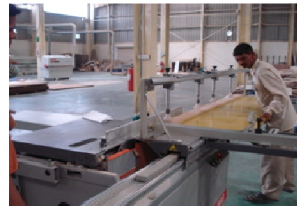
Trimming off edges
