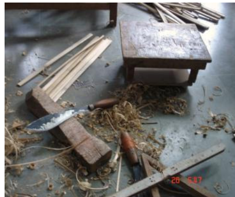
Cutting bamboo in to strips and finishing strips
