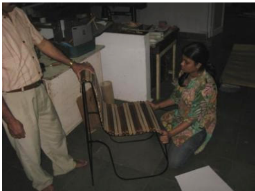
Putting mat on frame and fixing it.
