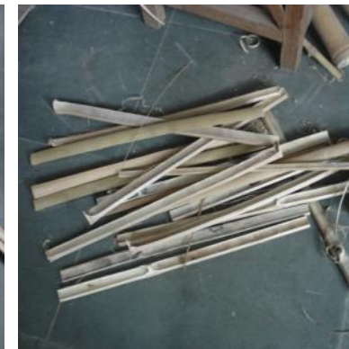
Cutting bamboo in to strips and finishing strips
