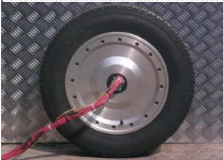
20kW hub mounted BLDC motor
