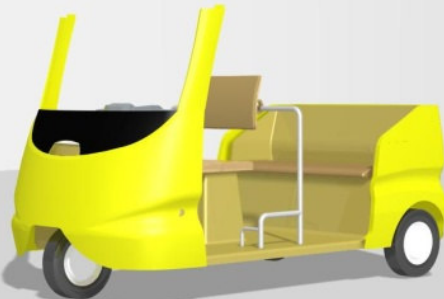
Bonding of the a pillars
