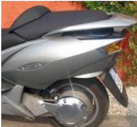
20kW hub mounted BLDC motor
