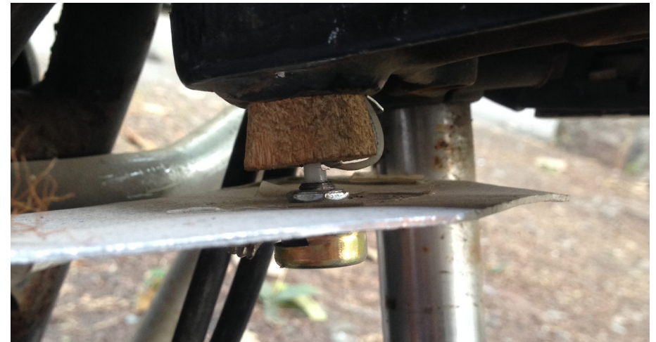
Figure 18. Potentiometer installation detail.
