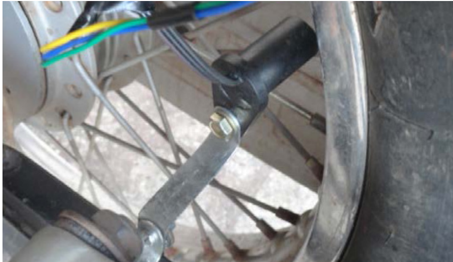
Figure 1. Hall effect sensor installation
