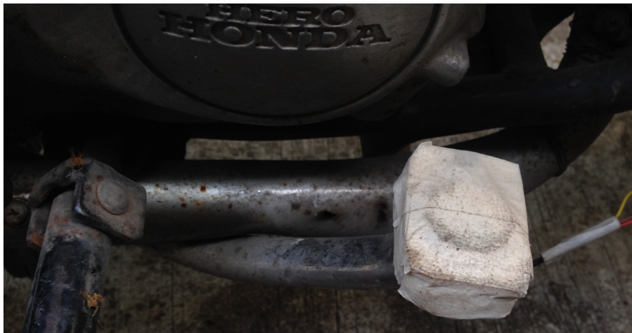
Figure 15. Pressure sensor and its installation on Bike
