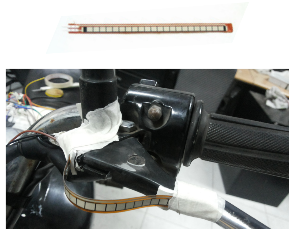
Figure 14. Flex sensor (top) and its installa
