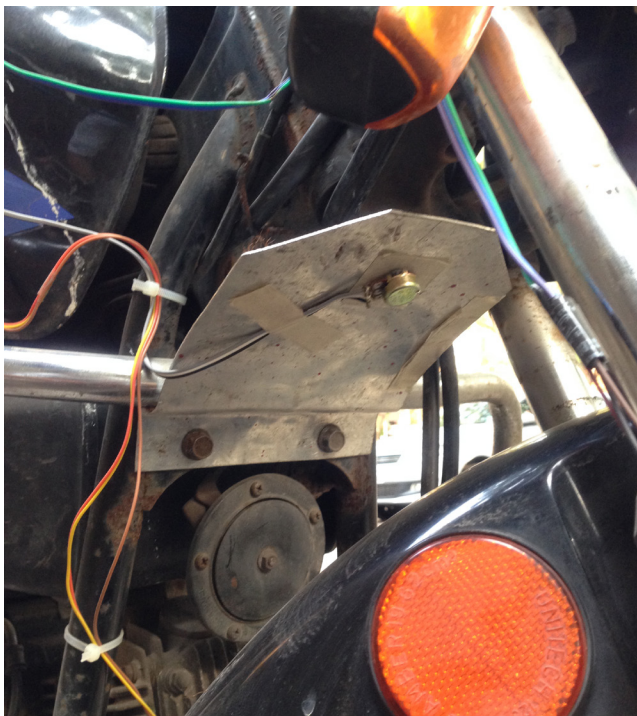
Figure 17. Potentiometer (top) and its installation in Bike
