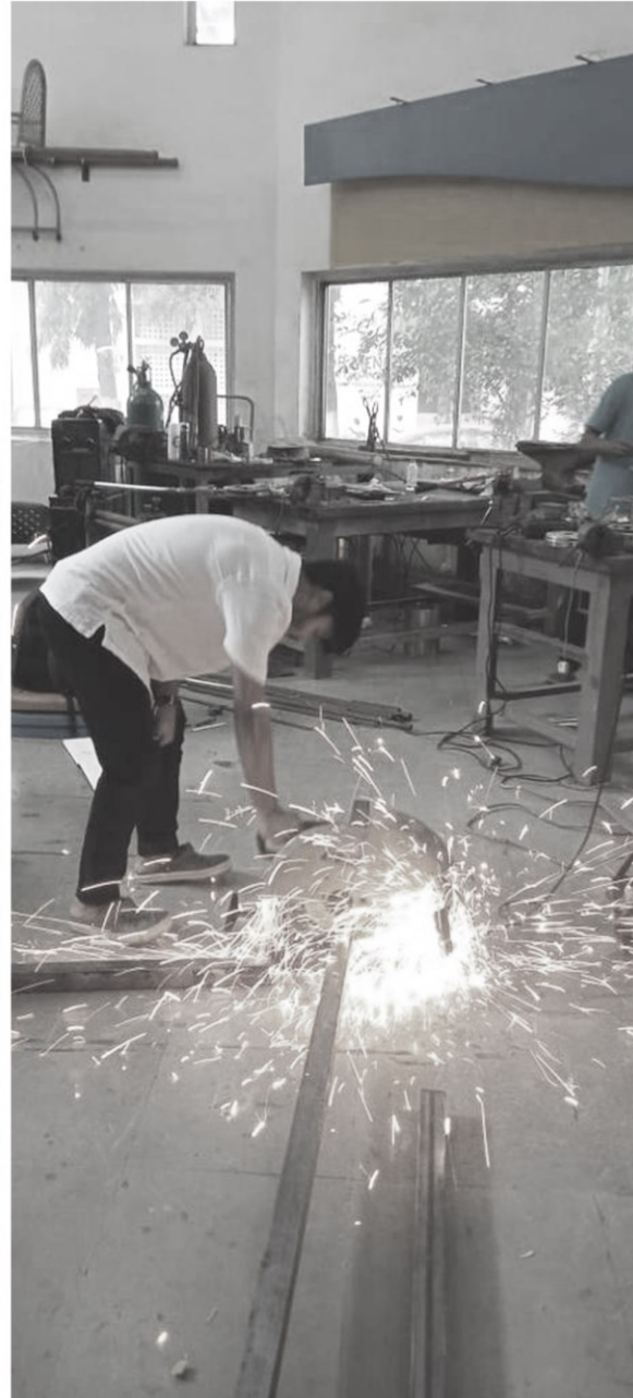
Fabrication of Solar Dehydrator Frame with 50mm Square M.S. Sections at PD Cell, IDC, IIT Bombay
