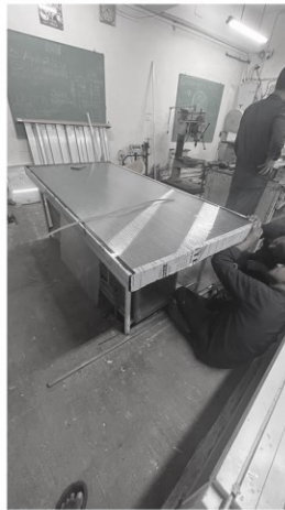
Fabrication of Solar Collector, that uses Aluminium Section Plate and Polycarbonate Sheets and Asawa Insulation sheet, thanks to Prof Mane . Fabricated at Heat Pump Laboratory, IIT Bombay.
