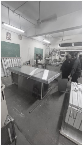
Fabrication of Solar Collector, that uses Aluminium Section Plate and Polycarbonate Sheets and Asawa Insulation sheet, thanks to Prof Mane . Fabricated at Heat Pump Laboratory, IIT Bombay.
