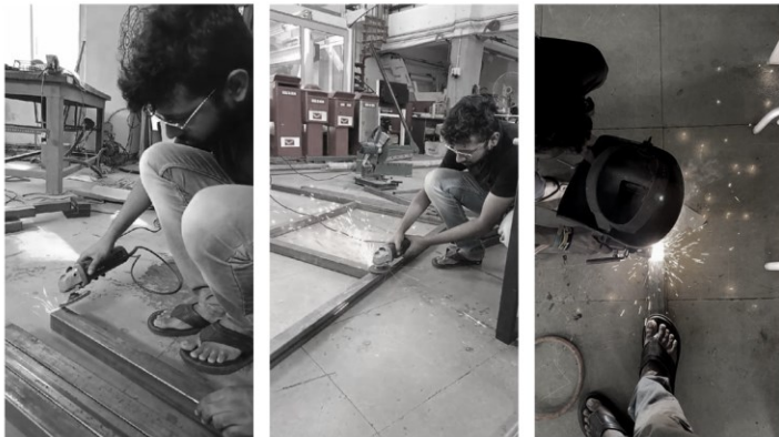
Fabrication of Solar Dehydrator Frame with 50mm Square M.S. Sections at PD Cell, IDC, IIT Bombay
