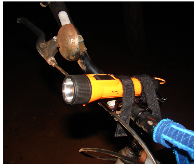
universal torch holder that can be fastened on the handle.
