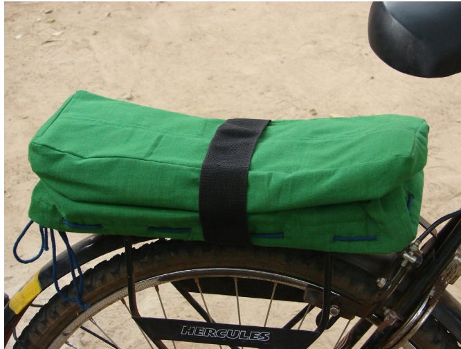
Saddle bag that can be folded and it becomes a seat for the pillion rider.
