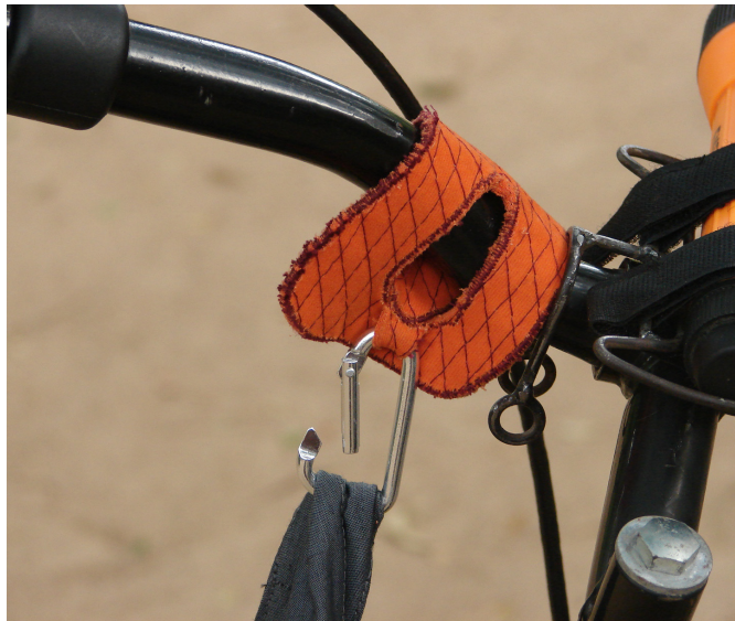
Universal hooks that can be attached at various points on the bicycle. Hooks can be used to hang things.
