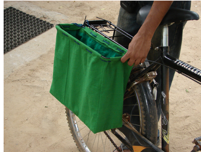
Saddle bag that can be folded and it becomes a seat for the pillion rider.
