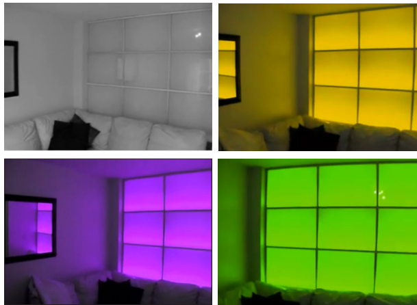
Image 48 Changing colour wall : This changing colour wall consists of wall modules which are backlit and programmed to change colour constantly
