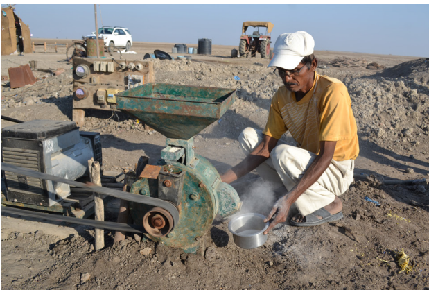
When not in use, the motor is connected to a grinder for grinding wheat and pulses
