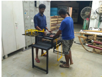
2. Place the mould on tray
