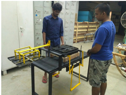
1. Slide tray under the mould
