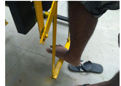
5. Press the foot pedal to lift the mould
