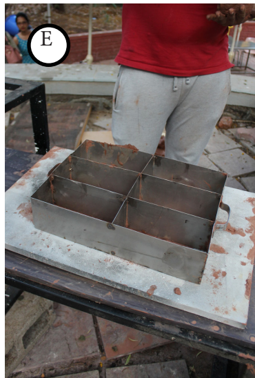
Aligning or lubricating the mould
