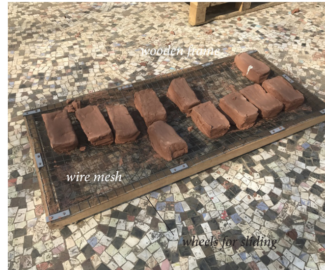
Fig : 64 (modification of mesh tray)
