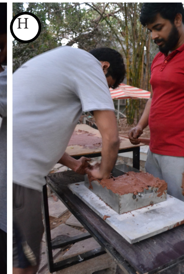
Pressing the excess mud
