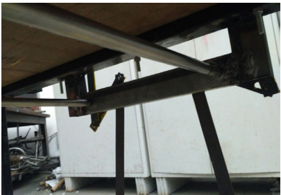
6. Connecting shaft turns both linkages together
