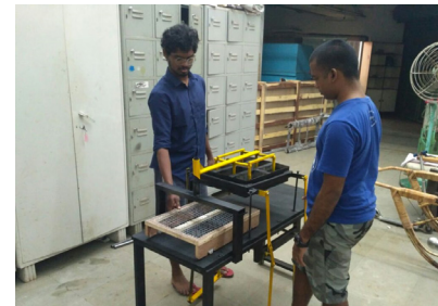
9. Tray is transferred for drying
