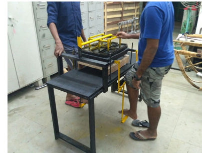
4. Rotate the cover on the mould
