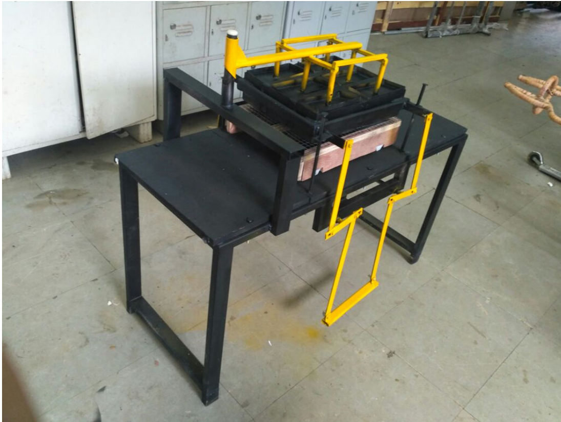
Fig : 73(Final Prototype of the brick moulding machine without the mud loading bay)
