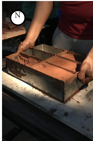
Lifting the mould up
