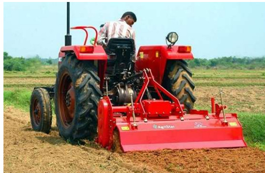
Rotavator to pulverise the soil
