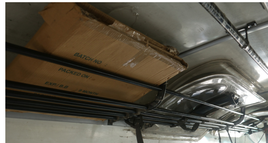
No proper mountings for the placement of equipment like shield, bullet proof jacket
