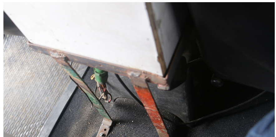
Walky talky stand mounted on the floor which act as a obstruction on the way.
