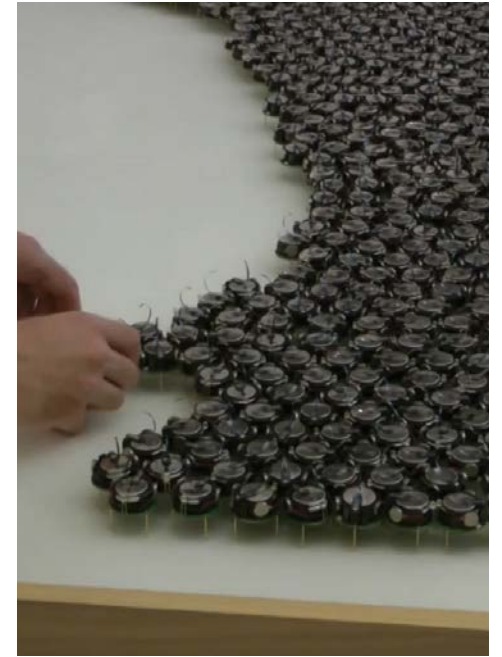
Img 14- Self assembly system
