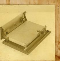
Place chassis on bottom plate and slide it back wards so that pins on the bottom end pieces of the front plate (attacked to chassis) slide into the corresponding holes in the bottom panel and the back of the
