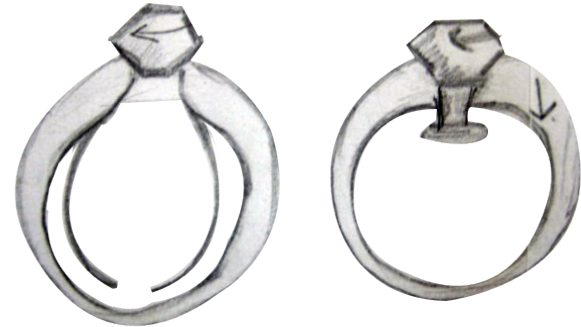
Mechanism to adjust the diameter of the ring using flanges (left) and screw (right)
