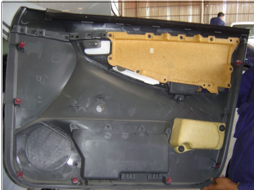
Internal panels used in automobiles are also made of structural polypropylene
