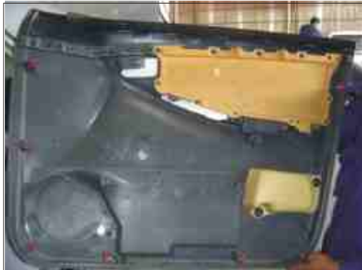
Internal panels used in automobiles are also made of structural polypropylene and are fit onto the inner metal body using plastic lugs.
