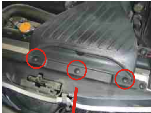
Internal panels used in automobiles are also made of structural polypropylene and are fit onto the inner metal body using plastic lugs.
