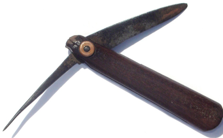
Fig. 3.11: A foldable stylus called pen knife. ( Image source: Pulavar Chockalingam )
