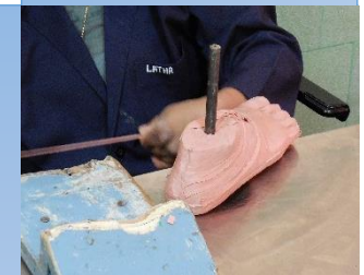
Entire block is covered with multiple layers of rubber
