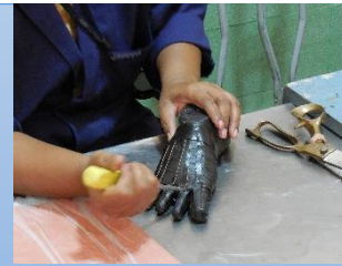
Another coating of resin layer is added
