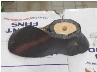
Wood block is cut and pasted with foam sheet
