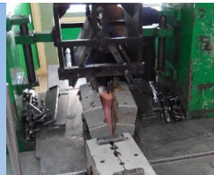
The dye is closed and pressed at a high pressure
