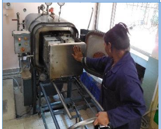
The dye is then heated up to 120°C
