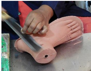
The foot is removed the from dye and extra pieces of rubber are cut
