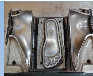
Block is placed inside a metal dye
