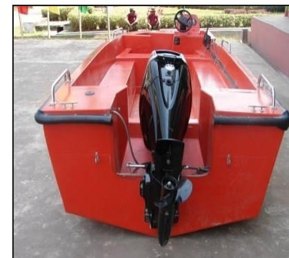
FRP boats (40 HP motor, carrying capacity: 30 people, Need to be transported in trucks)
