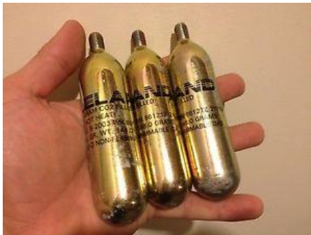
Fig. 5.23: \text{CO}_2 Cylinders used in life jacket for Inflation
