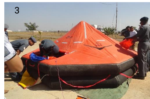
After 30 mins. The entire tube frame will get inflated
