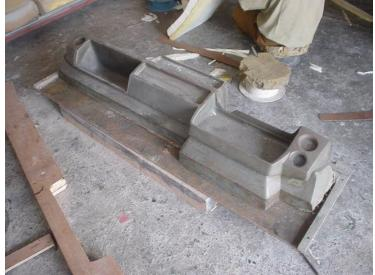
Mould is made around the pattern in FRP and is reinforced with m.s. square pipes. The pattern is then removed.
