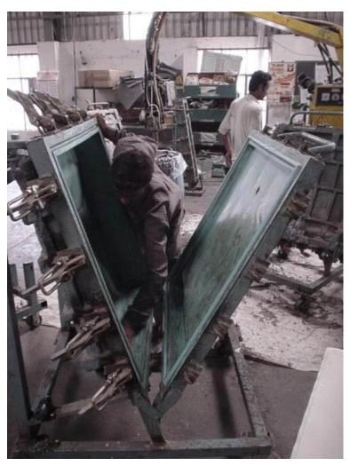
A mixture of Polyol 477 DOW and Isocynate 113 DOW is mixed in desired proportions and poured in the mould
