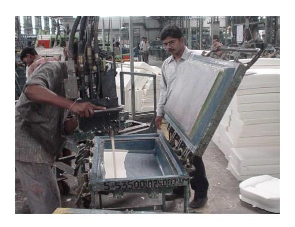
• The mould is then closed and the foam is allowed to expand.
