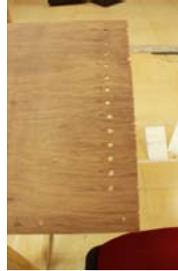
image99 graduations for various heights of steering wheel from the ground
