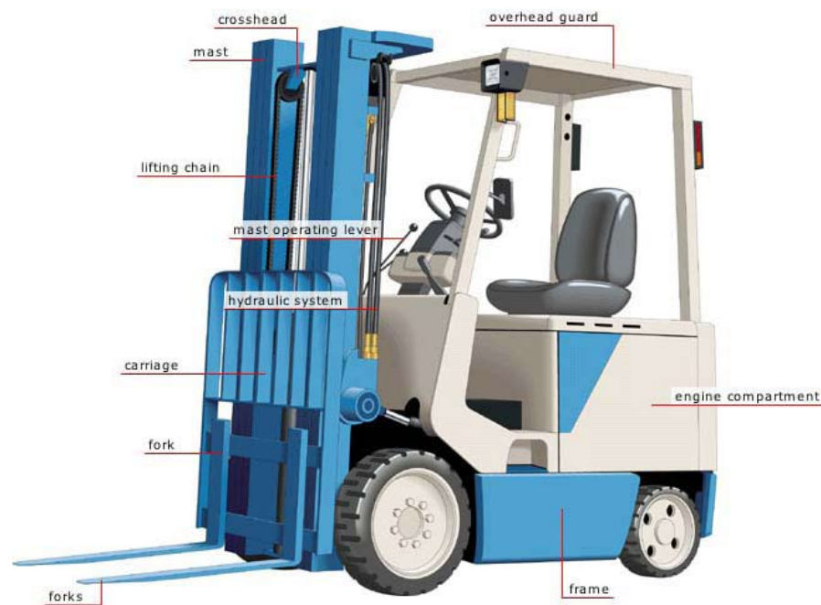
image2: parts of counterbalance electric forklift [1]
