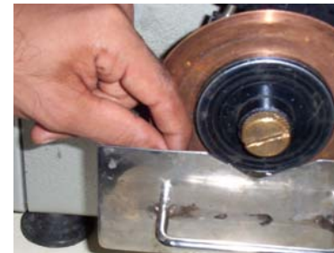
4. Setting the thickness of the slice
