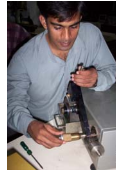
4. Setting the thickness of the slice
