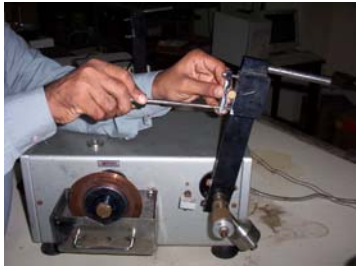
1. Fixing the work piece in the vice
