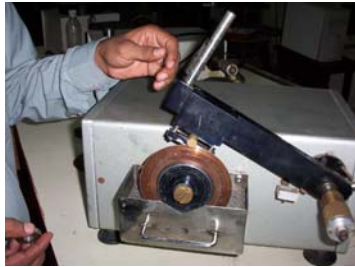
2. Getting the work piece in contact with the cut-of wheel
