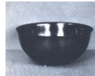
'Sinking bowl' type of water clock
