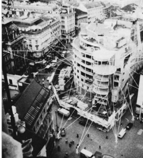
Figure: Construction of 3D images from photographs using Lambert's Space Resection
