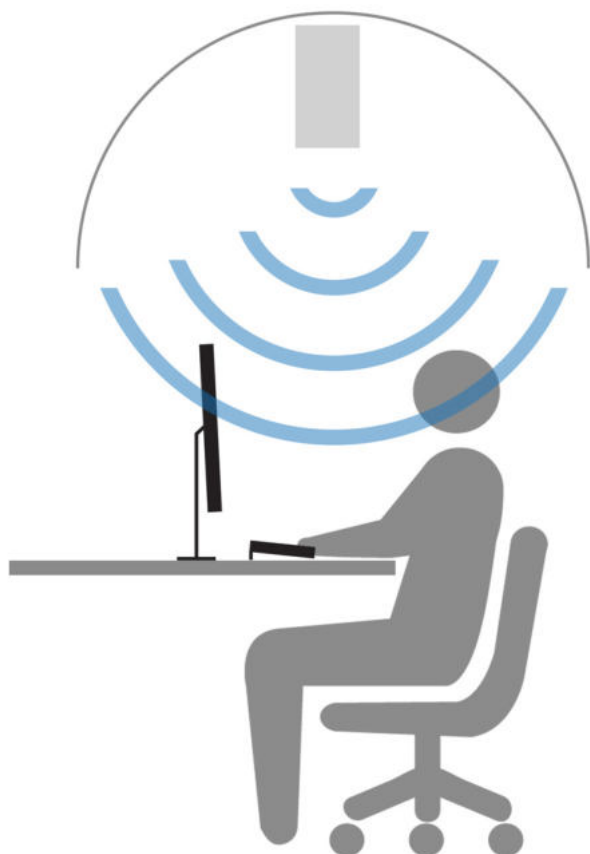
A user sitting under a sound dome that produces anti-noise
