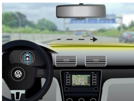
The LED strip shows the lights running in the direction of the turn
