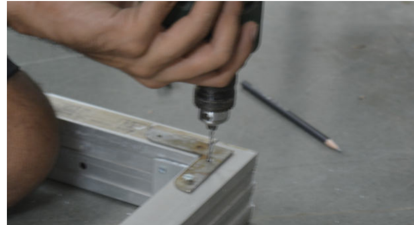
Drilling through the flat L-angle to make give more reinforcement at the corners
