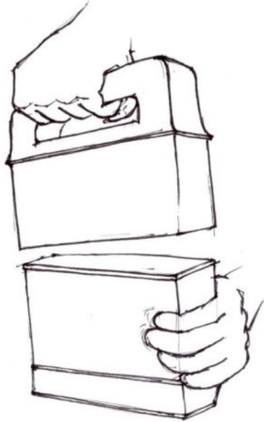
Lamp being detached
