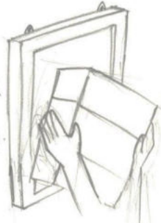
(ii) The lights being un-docked from the panel
