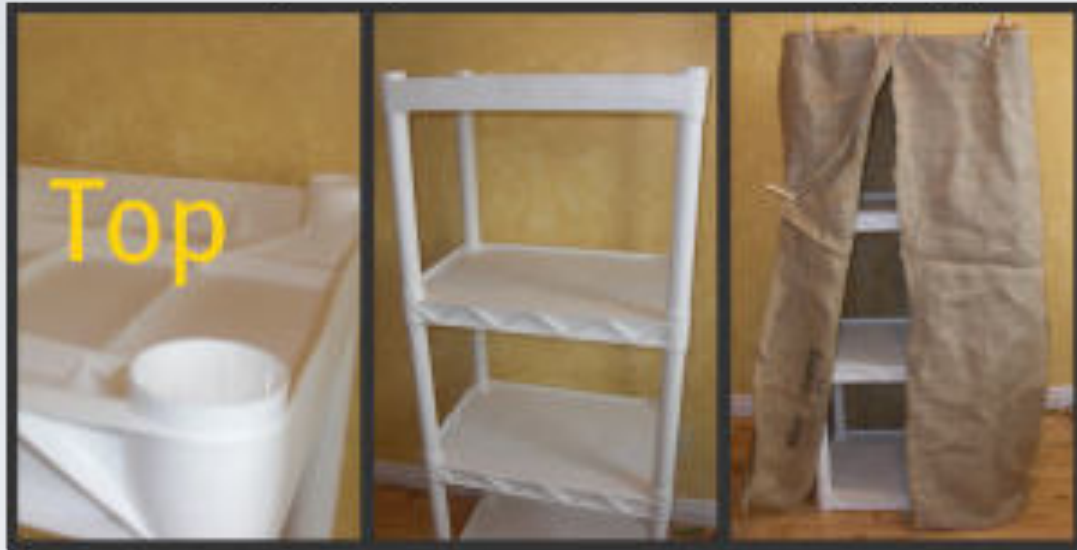
Evaporative cooler fridge (using continuous water dripping)
