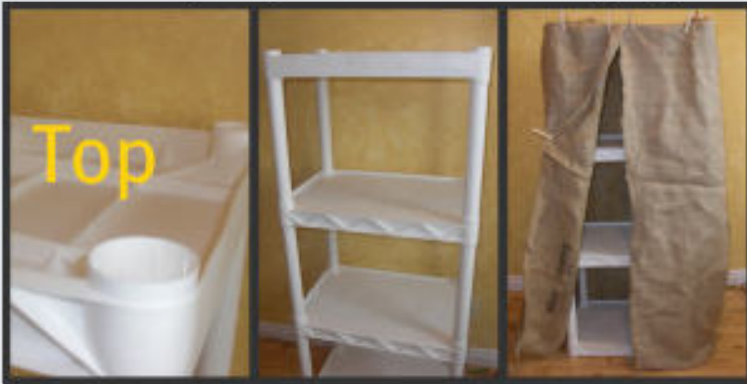
Evaporative cooler fridge (using continuous water dripping)
