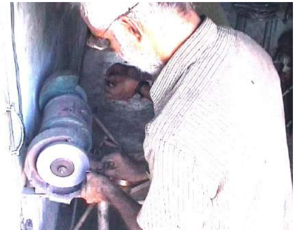
Mr. Sawant grinding the rim binding tool to shape
