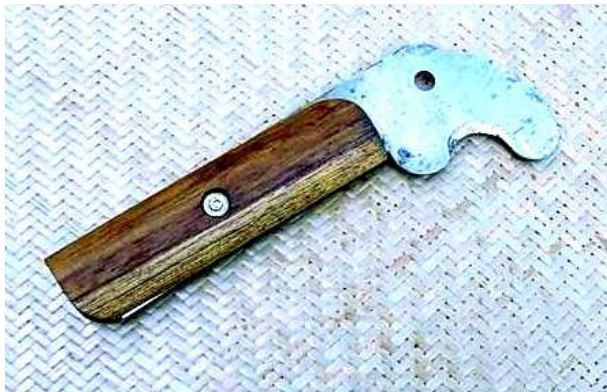
Cane scrapper developed at IDC
