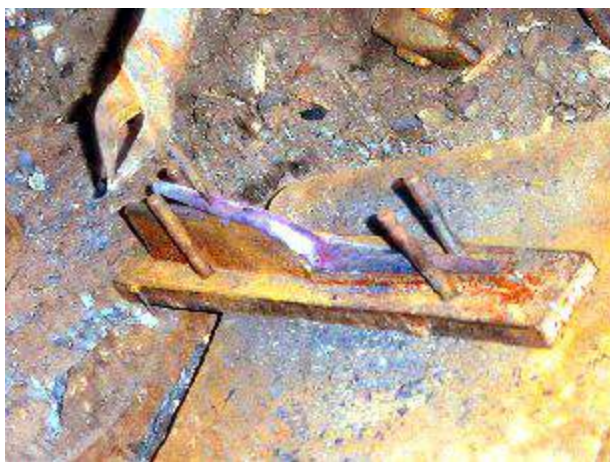
shaping a laser cut blank into propping knife by the local smith
