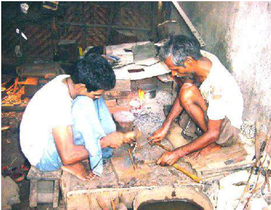
shaping a laser cut blank into propping knife by the local smith
