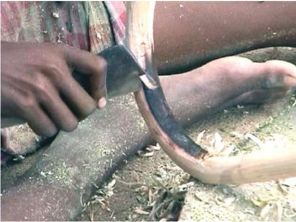
Cane being scrapped at the inside curvature with a dhau at Andaman Nicobar Islands
