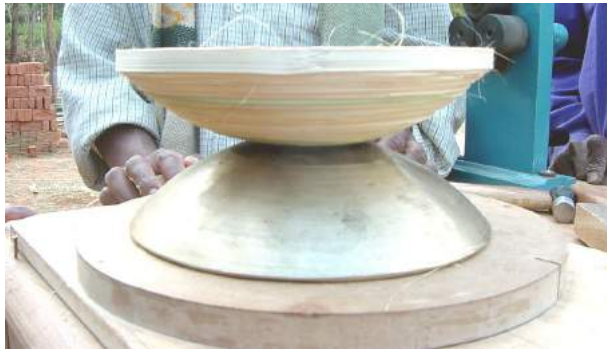
Bowl made of coil technique using a local thali as mould
