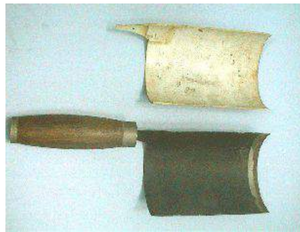
plastic mock-up of chinese rounded scraping knife made and given to local smith
