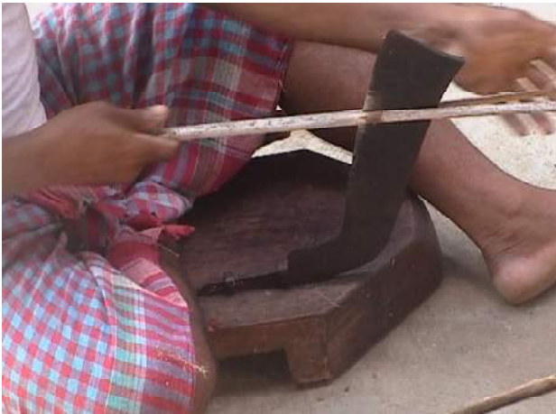
Cane split in Andaman using tool in Tripura style
