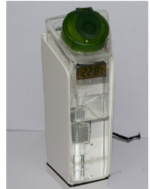
Mockup featuring seperate cooling unit temperature display and peltier on sidewall
