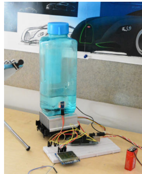
Single chamber with peltier on wall
