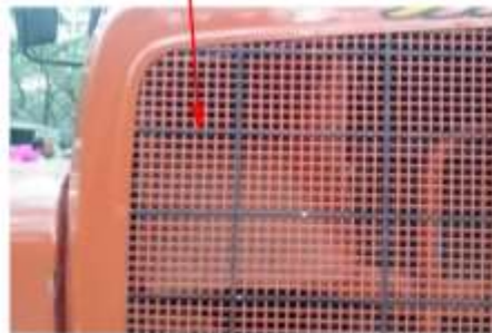
Vent for air duct to cabin for ventilation
