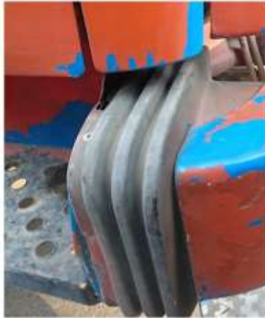
Rubber bellow is between Footrest and bumper
