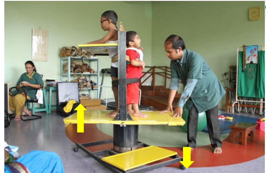
Fig.5.1 the physiotherapist in a bad posture, exerts force at the end of the platform which requires more force to compress the spring (designed to sit and exert force on the area near the cylinder)
